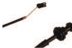
Choke Cable, Yamaha Gas G2/G9 Length: 34". OEM: J55-F6331-01. CBL-005
