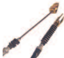
Brake Cable, Passenger, Yamaha G1A+E/G2E/G9E Length: 48½". OEM: J56-F6351-01-00. CBL-002
