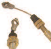
Accelerator Cable, E-Z-Go 89-94 2 cycle Length: 56". OEM: 22334-G1. CBL-027
