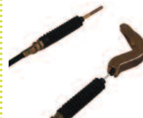
Forward/Reverse Cable, E-Z-Go Workhorse 96 & up Length: 45¼". OEM: 72341-G01. CBL-019
